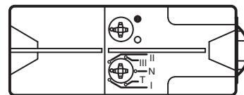
You need not turn the switch into T-position again, when changing the contrast recognition value during operation. For sensor operation in contrast recognition mode, the stability control value must be at least 2.5 (see curve relative received light strength).
